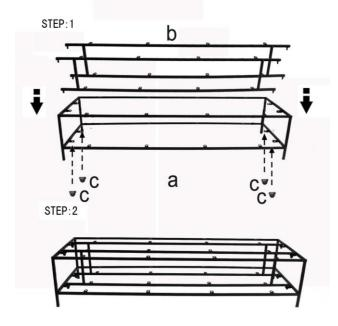
Step 1: Place the bottom (A) display on a leveled surface. Take both bars (B) and attach them to the holes found in the middle of the display, use 1 screw (C) per side tighten screws using the wrench (D). Make sure that all holes are on the same direction as shown in the diagram above.
